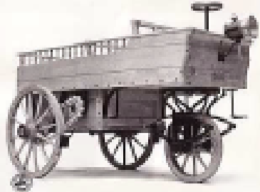
1-cylinder Hydrogen Vehicle by Lenoir, 1860
